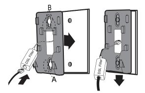
3. Align and place the telephone base on the wall mount bracket, and then connect the power adapter.
