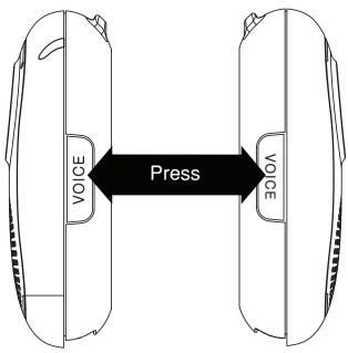
Press **VOICE** on either side of the pendant when the telephone is idle. After you hear a beep, say your command to the pendant.
